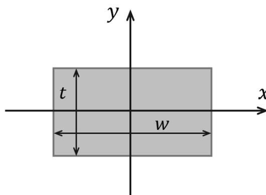
Fig. 2 Schematic illustration of the cantilever beam cross-section.
