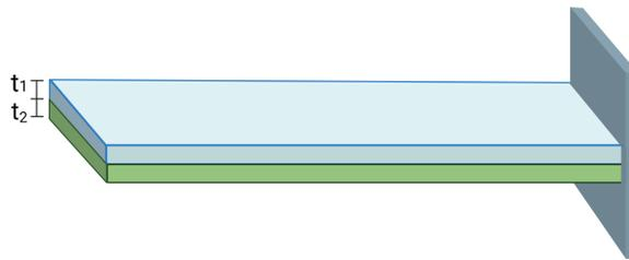
Figure 5: Double layer beam (Upper layer is metal X. Lower layer is silicon.)
