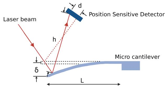
Figure 3. Illustration of the optical leverage setup.
